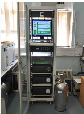
A Picarro analyser and an Essex Air Sampling Canister at the University of Bristol, UK.
