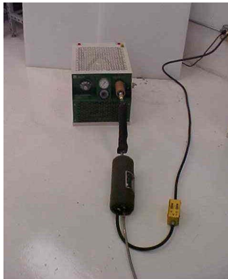
Figure 4.3 Purge Kit Setup
