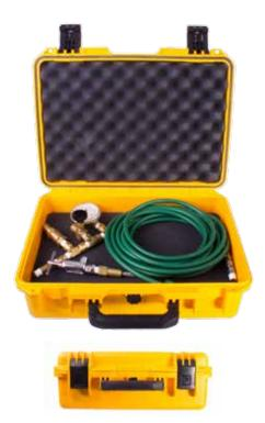
The High Pressure Fill Kit connects the OGL or OGS with a high pressure oxygen compressor to fill high pressure cylinders with 93% USP oxygen. The kit includes a 20' low pressure oxygen hose and a 4' high pressure braided hose with a relief valve, manual vent valve and pressure gauge. The high pressure oxygen compressor is not included. Items are packaged in a protective storage case.
