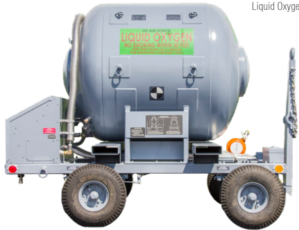
500 Gallon Liquid Oxygen Trailer
