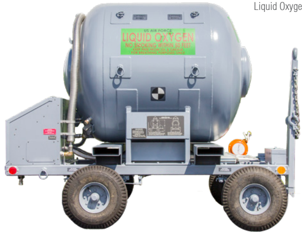
500 Gallon Liquid Oxygen Trailer
